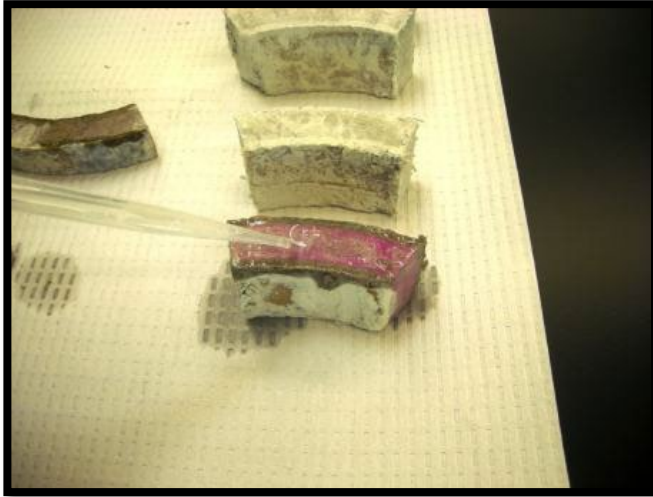
Typical Application of Phenolphthalein to a sample of AC pipe
