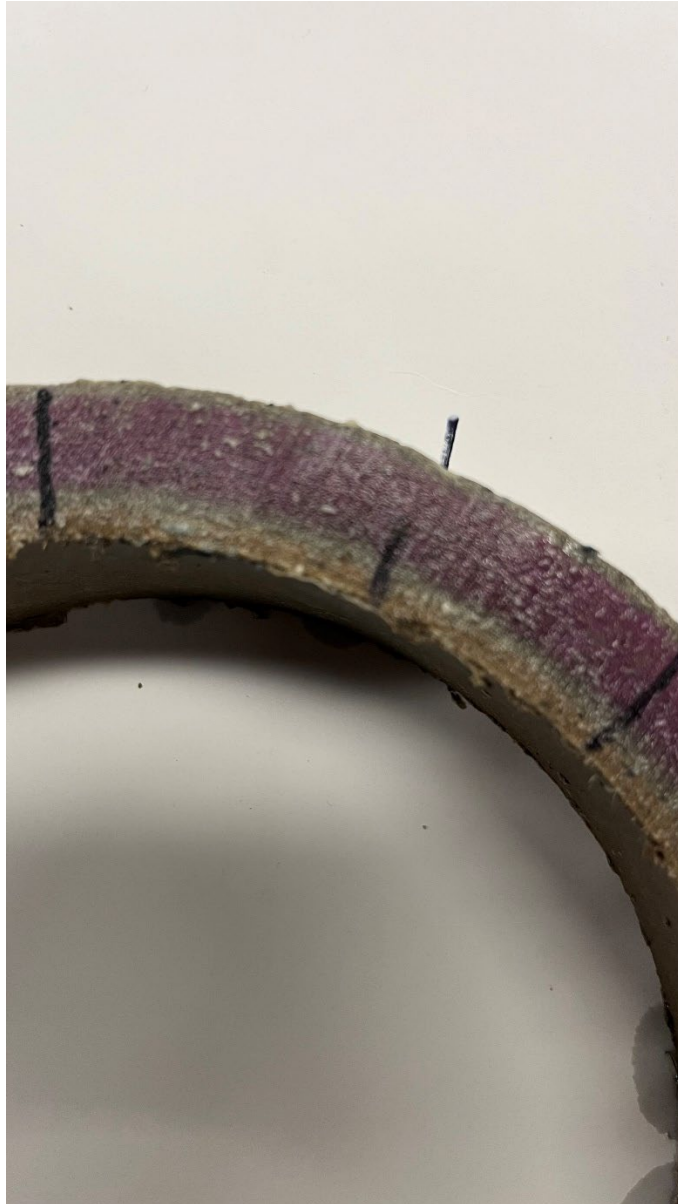
Photo 2 –6-inch AC Pipe segment close up several minutes after staining with phenolphthalein
