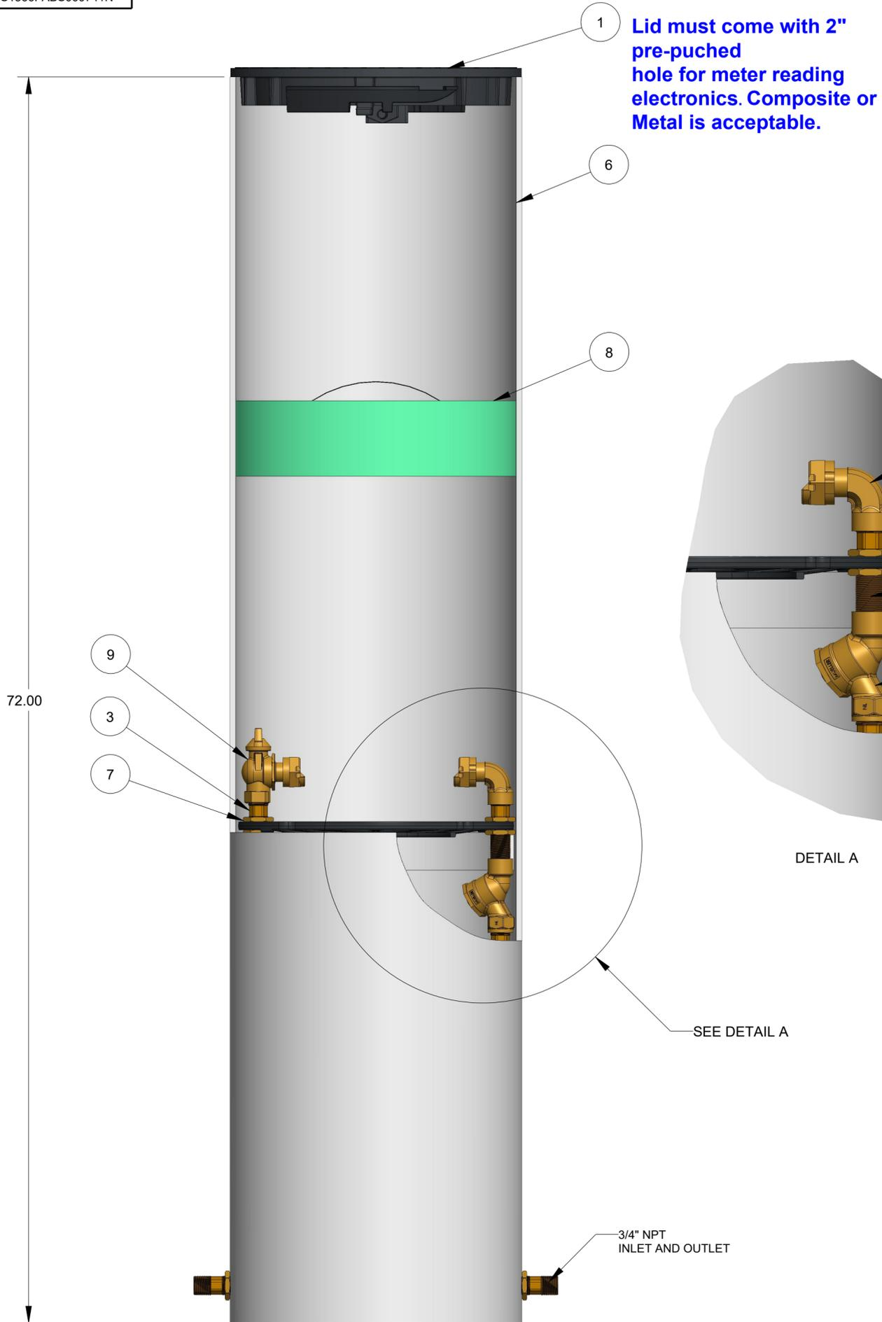
1 Lid must come with 2" pre-punched hole for meter reading electronics. Composite or Metal is acceptable.
